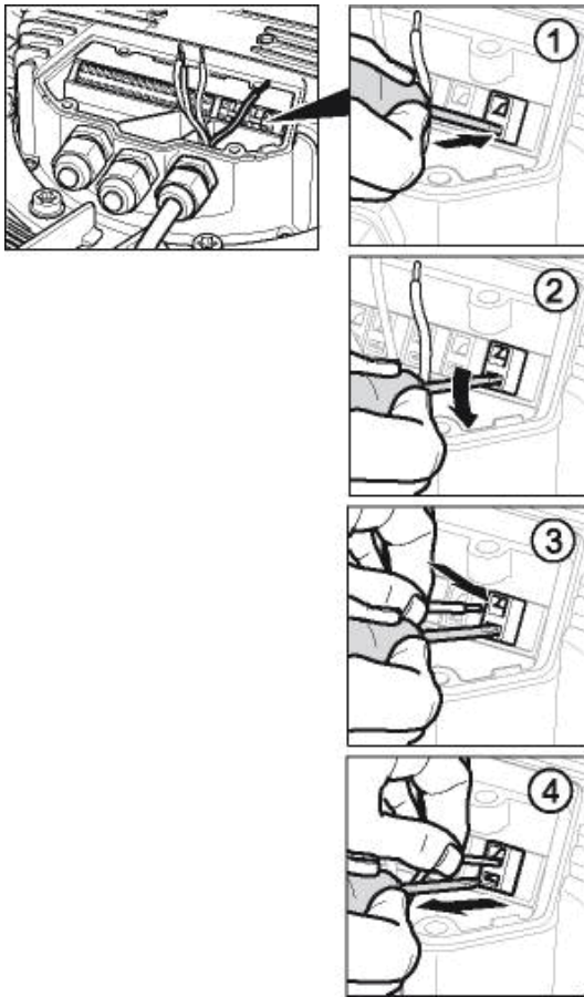
Fig. 2: Connecting wires to terminals
